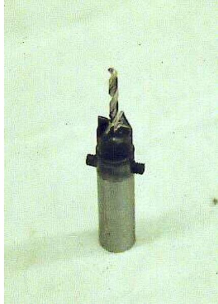
spot faced, with a homemade spot face/drill
