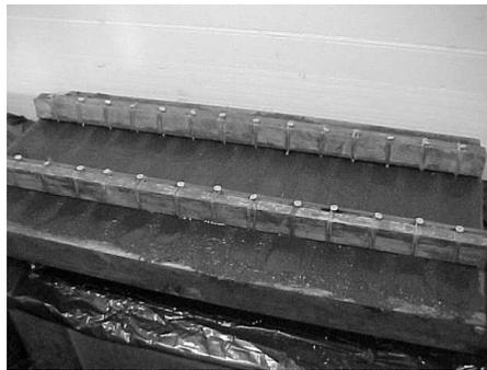
12. Let set for 24 hours and remove all the rubber bands from the form and gently remove the sides and starting on one end remove one end, one tie, one spacer, one tie, another spacer, another tie, etc.
